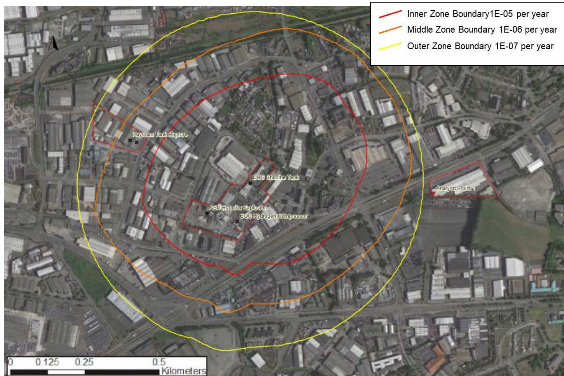
Figure 7-1 Individual Risk of Fatality Contours for BOC Gases Ireland and Kayfoam Woolfson
