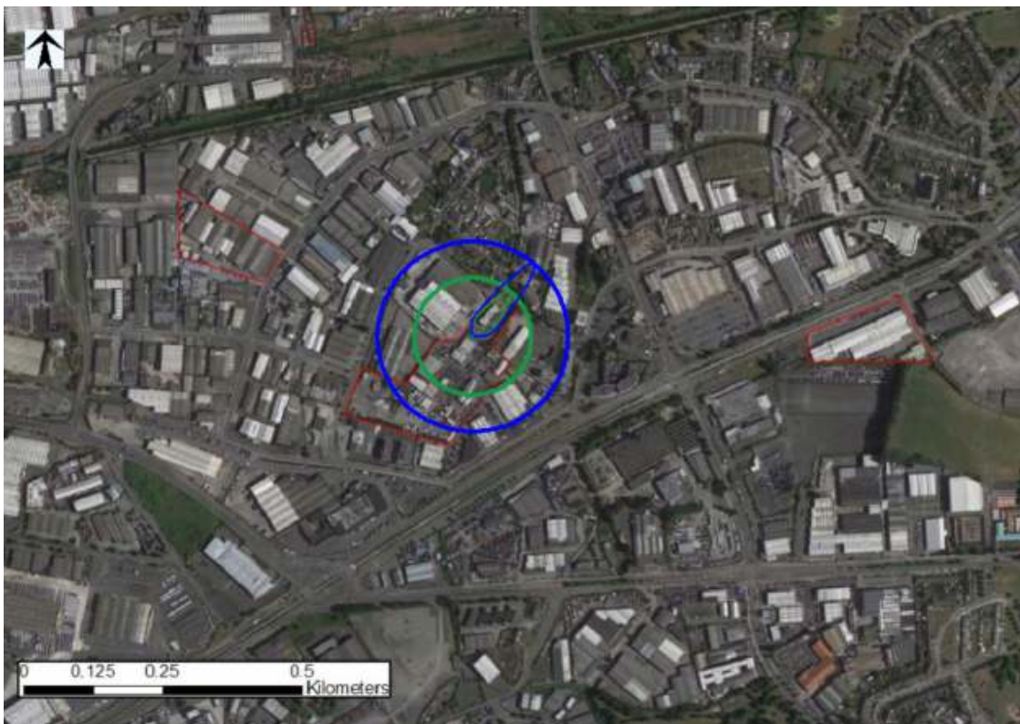
Figure 5-2 Chlorine Drum Drop 5 min release: SLOT and SLOD DTL Outdoor Contours (Category D5)
